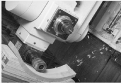
Eight 5 Axis CNC: Chair parts design and production
